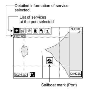
Figure 2-8 Plotter display showing Nav-Charts™ port service display
